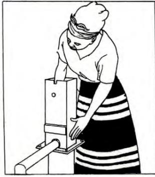
27. Make sure the foot valve is in place by pushing the rods at arms length down the borehole.
