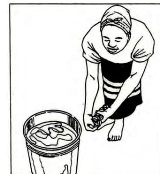
22. Wash the foot valve, plunger and rods. Use only clean water.
