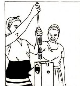
17. Remove all the rods, the fishing tool and the foot valve.
