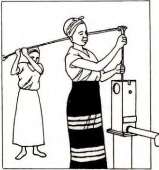
13. Disconnect and remove all rods. Remember to keep the rods in the same order. The last rod taken out should be the first rod put back.
