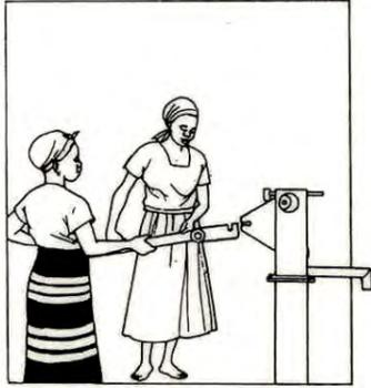
7. Raise and withdraw handle. Take care! As you remove the handle make sure the bush bearings and pin do not fall out as they may break on the floor.
