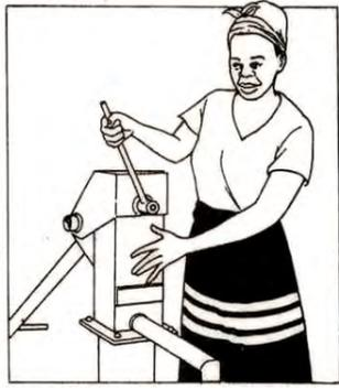
2. Loosen the pump head cover bolt
