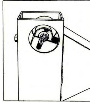
34. Push the handle down so that the slots engage in the hanger. Ensure that the hanger pin has slid to the bottom of the slots. Remove the spanner.
