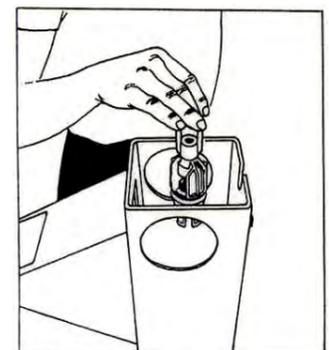
23. To reassemble the pump, first drop the foot valve down the borehole. Make sure the hook is upwards
